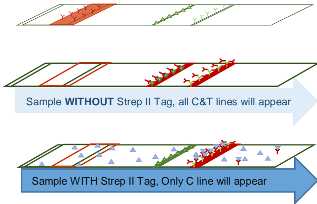
Figure 1. Diagrams illustrating competition LFIA. Top: Layout of an unused test strip. Middle: When a sample without Strep tag II is applied, four red lines will appear. Bottom: When a sample with enough Strep tag II is applied, one control line will appear. Y Gold labeled Anti-Strep Tag Antibody ▲ Test Line immobilized Strep Tag II tagged protein Y Control Line immobilized 2 nd Antibody ▲ Strep Tag II Tagged protein in sample
